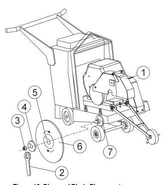
Figure 12. Diamond Blade Placement
